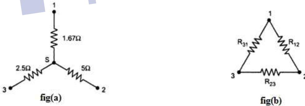
Solution: The equivalent delta for the given star is shown in fig(b), where
